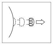
2. To input data, contact each terminal and the side face of the battery repeatedly with the tool until the desired data is shown in the calendar frame.
