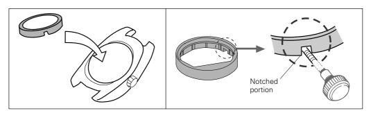
3. Put the edge of the battery under the installer.
