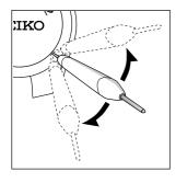
\* Do not pry the battery up. This will damage the movement.
