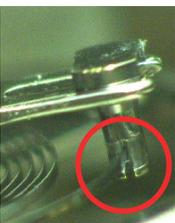
\* When assembling the BALANCE COMPLETE, pay great attention not to deform the balance-spring, especially at the second bend.
