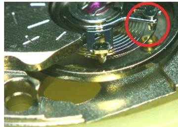
4) Push back the stud parallel to the slit of the STUD SUPPORT.
