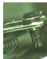
2) Rotate the STUD in order to align the position of the balance-spring passes through the center of the slot of the REGULATOR PIN.
